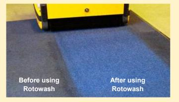
Rotowash brushes out dirts and particles trapped inside carpet which can't be removed through vacuuming, leaving a clean and bright appearance.
